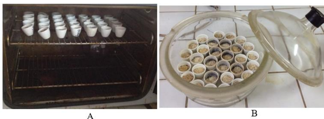
Fig. 4. Procedure for determining moisture and ash content A-Placing the crucibles containing the flour in an oven, B-Cooling in a desiccator
