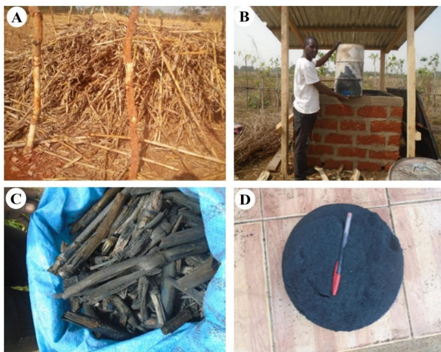
Fig. 3. Different steps of biochar production. A. Maize residues, B. Experimental system, C. Biochar produced, D. Fraction sieved at 2 mm to be used for incubation
